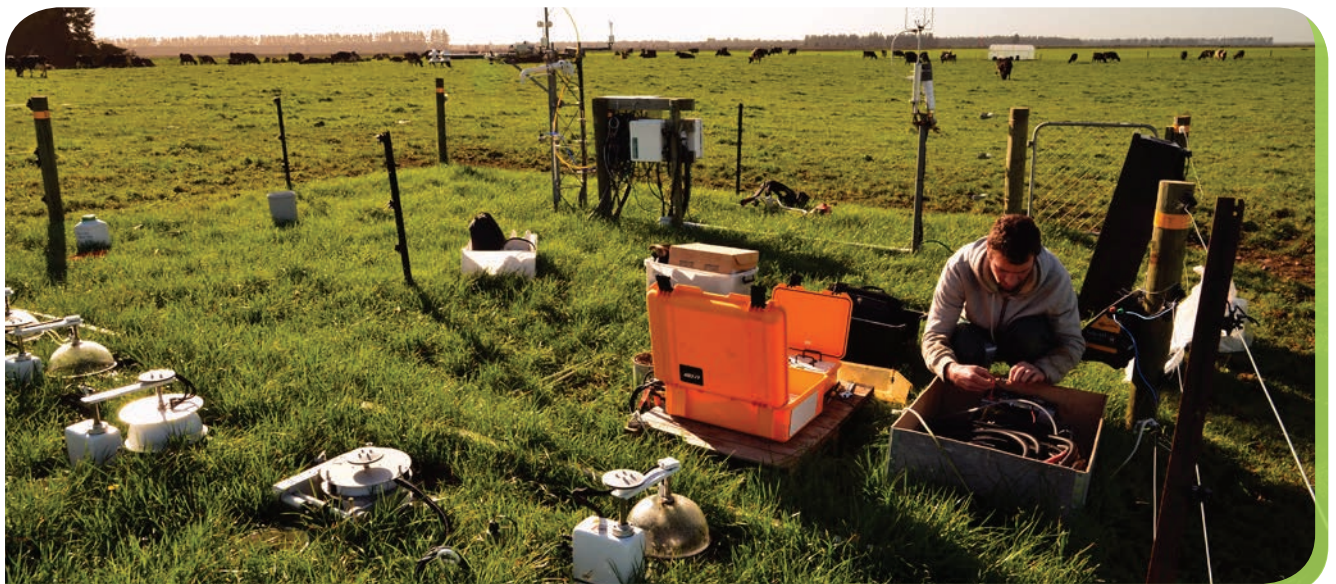
Continuous measurements of carbon exchange from pasture and soil using automated chambers. Photo by John Hunt.
